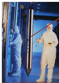
growing the silicon ingot
