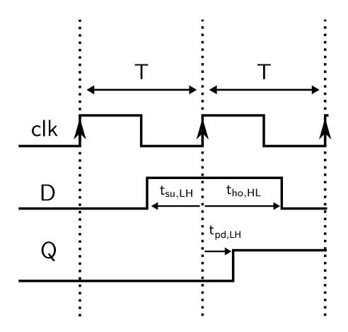
In the report, show the input and output waveforms from Cadence to demonstrate that your flip-flop circuit is indeed working. To do this, pick a setup and hold time that enables your flip-flop to sample the input value. Show that you can sample both high and low levels. Do not forget to include the output load capacitance in your schematic.
