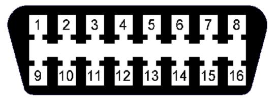
Pin 2 - J1850 Bus+ Pin 4 - Chassis Ground Pin 5 - Signal Ground Pin 6 - CAN High (J-2284) Pin 7 - ISO 9141-2 K Line Pin 10 - J1850 Bus Pin 14 - CAN Low (J-2284) Pin 15 - ISO 9141-2 L Line Pin 16 - Battery Power
