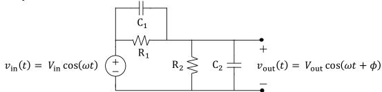
Determine the two relationships that are required between  $R_1$ ,  $R_2$ ,  $C_1$  and  $C_2$  so that  $v_{out}(t) = 0.1v_{in}(t)$  for all values of radial frequency  $\omega$ . That is, what relations are required so that  $\hat{V}_{out} = 0.1\hat{V}_{in}$  (i.e.,  $V_{out} = 0.1V_{in}$  and  $\phi = 0$ ) for all values of  $\omega$ ?
