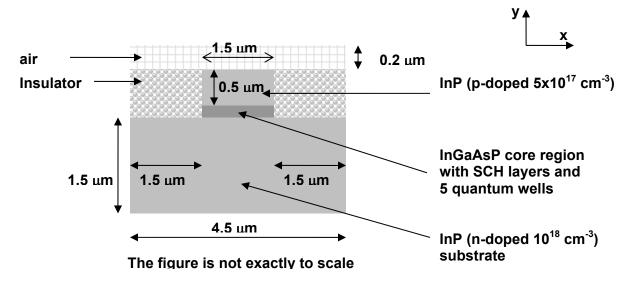
The thicknesses of various layers in the core region (SCH layers plus quantum wells) are shown in the figure below. The quantum well barriers and SCH layers have the same composition. The core region is undoped.
