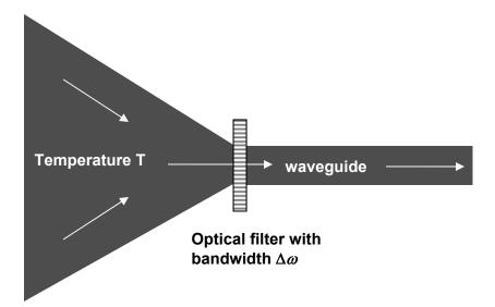
Radiation from some thermal source at temperature T is collected and channeled into a **non-interacting non-dispersive** waveguide. An optical filter with transmission bandwidth  $\Delta \omega$  centered at  $\omega_0$  is placed in front of the waveguide. The filter only allows incoming photons that have frequencies within this transmission band to pass. It therefore makes sense to expand the field operator inside the waveguide in only this bandwidth  $\Delta \omega$ , as shown below,
