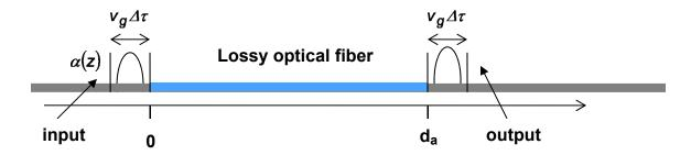
I have adjusted the spatial co-ordinate system so that the zero of the co-ordinate system is the beginning of the lossy region of the fiber. The input photon number operator is defined as:
