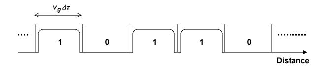
The data rate is clearly one bit of information per  $\Delta \tau$  seconds, or  $1/\Delta \tau$  bits/sec. In state of the art commercial optical systems data rates are between 10-40 Gbits/sec, so the duration  $\Delta \tau$  is between 100 ps and 25 ps.
