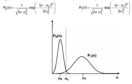
These probability distributions are sketched in the figure above. A system designer must decide upon a threshold photon number  $n_c$  so that if the number of photons counted in any one bit interval of duration  $\Delta \tau$  comes out to be larger than  $n_c$  then a logical 1 is declared, and if the number of photons counted is smaller than  $n_c$  a logical 0 is declared. These decisions are made by electronic circuitry in the receiver.
