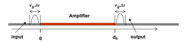
I have again adjusted the spatial co-ordinate system so that the zero of the co-ordinate system is the beginning of the amplifier. The input photon number operator is defined as:
