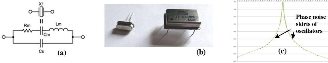
Fig. 2. Crystal oscillators based on piezoelectric quartz crystal vibration: (a) Circuit symbols and van Dyke equivalent circuits; (b) Hermetic packaging to reduce the influence from ambient air; (c) Typical resonator response with Q > 1,000 .
