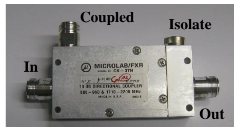
Fig. 2. Microwave/RF directional coupler based on transmission lines: (a) Schematic where P1 \leftrightarrow P2 is about -0.5\text{dB} (top bidirectional and bottom directional) and P1 \rightarrow P3 is about -10\text{dB} and P2 \rightarrow P3 is about -50\text{dB} (directional); (b) A commercial sample with dual bands of operations.
