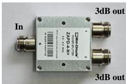
Fig. 1. Simple broadband signal splitter based on microwave transmission lines. Detailed waveguide structures, instead of lumped LC elements, are used to create the splitting functions and impedance matching. Most often the two output ports have 3dB loss due to splitting, i.e., half of the input power going to each output port. There can be an identical phase shift to the two output ports.
