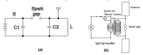
(a) In Fig. (a), what is the approximate frequency of emission (hint: the resonant frequency when the spark is generated)? (5 pts)
