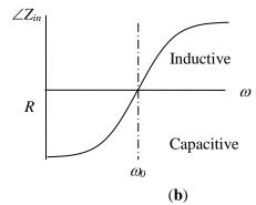
5. (**Resonator as impedance transfer**) The resonator can be used to transfer resistance to make it seem larger or smaller at the resonant frequency. An example for "**impedance up conversion**" is shown below, and is called the "L-section". This is another way to match the impedance to or with the transmission line, as shown in the right figure.
