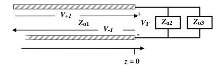
As all transmission lines here are considered with infinitely long, the impedances looking into lines 2 and 3 are just  $Z_{o2}$  and  $Z_{o3}$ .
