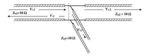
(a) Looking to the right of the dashed line, the two output transmission lines can be represented as lumped impedances so the equivalent circuit becomes as shown below. Find the amplitude  $V_{-1}$  of the reflected wave in terms of the input wave amplitude  $V_{+1}$  (5 pts) and find the fraction of the input power that is reflected. (5 pts)
