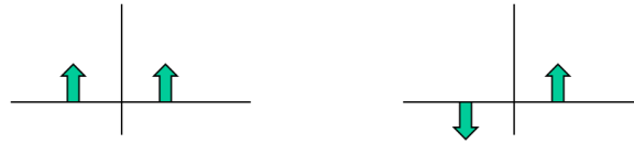
Fig. 8.5. Spectral representation of real signals in cosine and sine functions. Notice that the phase offset has been absorbed into t . However, with the same t , cosine and sine are 90^\circ apart.
