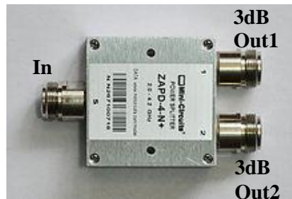
Fig. 7.1. Microwave or RF power splitter based on transmission lines.
