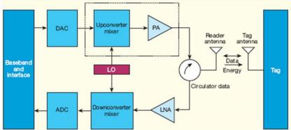
Block diagrams for RFID. Questions 3 – 8 all used the same parameters and conditions.
