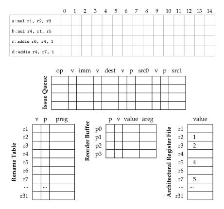
We can use a table to compactly illustrate how IO2L value-based register renaming works. We show the state of the RT and ROB at the beginning of every cycle.
