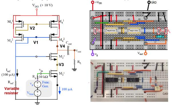
Note that the output is AC coupled through a 0.1  $\mu$ F capacitor. Verify that  $R_{ref}$  should be around ~69 k $\Omega$  in order to get  $I_{ref}$  around ~100  $\mu$ A. Actual values of  $R_{ref}$  can vary from chip to chip. Use a variable resistor as  $R_{ref}$ . After you have connected the circuit verify that  $I_{ref}$  is indeed ~100  $\mu$ A. Select  $V_{bias}$  to be close to ~1.25 V.
