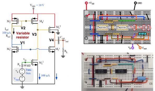
b) Select a 1 kHz sine wave on the function generator. Set the DC voltage offset on the function generator to the chosen value for  $V_{bias}$ . Set the function generator to a 5 mV peak-to-peak AC amplitude (really small). Remember to Recall ECE2100Setup and enable external trigger on the scope. Both scope channels should be AC coupled. Connect everything (except the load resistor).
