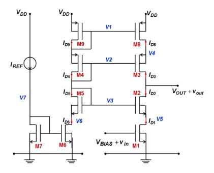
a) Assuming that the resistance looking into the PFET biasing source on top of the cascode is very large, what value should one choose for the width  $W_1$  of M1 such that the transconductance of the cascode amplifier is around 1 mS?
