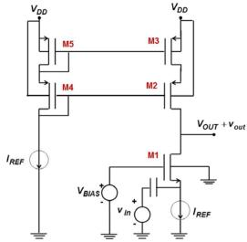
a) Find the open circuit voltage gain  $A_v = v_{out} / v_{in}$ .
