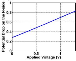
When V equals 1.31 Volts, the potential drop on the N-side becomes equal to 0.83 Volts.
