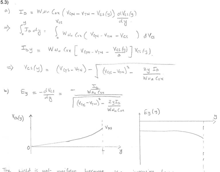
The field is not uniform because the inversion layer charge density is not uniform along the channel. Is the inversion layer charge density decreases going towards the drain end, the field increases, but the product gives the constant current (i.e. independent of position).
