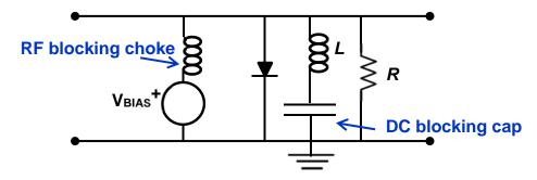
The inductance of the inductor is L = 5 nH. The dopings in the diode are:  $N_a = 10^{14}$  1/cm<sup>3</sup> and  $N_d = 10^{16}$  1/cm<sup>3</sup>.
