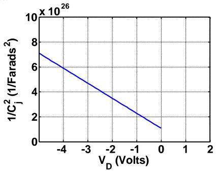
a) From the data shown above, figure out the built in voltage  $\phi_B$ .
