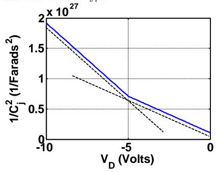
You can see that for values of  $V_D$  less than -5 Volts, the data changes slope (the magnitude of the slope increases by a factor of two).
