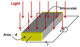
Consider a device consisting of a piece of P-doped silicon ( $N_a = 10^{15} \text{ cm}^{-3}$ ) with an area A equal to 1.0 sq -  $\mu$ m and length L equal to 1  $\mu$ m. The electron and the hole mobilities are 1000 and 300 cm<sup>2</sup>/V-s, respectively. The minority carrier lifetime  $\tau_n$  is 1  $\mu$ s.
