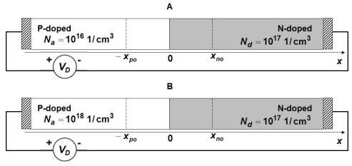
a) At  $V_D = 0$  Volts, which diode has the wider total depletion region width  $(x_{no} + x_{po})$  and what is its value (in microns)?
