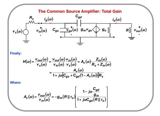
The Common Source Amplifier: Poles and Zeros of the Total Gain  $H(\omega) = \frac{A_{v}(\omega)}{1 + j\omega [C_{gs} + C_{gd}(1 - A_{v}(\omega))]R_{s}} = \frac{H(0)(1 - j\omega\tau_{3})}{(1 + j\omega\tau_{1})(1 + j\omega\tau_{2})}$
