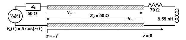
The circuit is operating at a frequency of 1.0 GHz. At the load end of the circuit there is a 70  $\Omega$  resistor in series with a 9.55 nH = 9.55x10<sup>-9</sup> H inductor. The length of the transmission line is such that:
