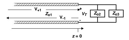
Find the amplitude  $V_{-1}$  of the reflected wave in terms of the input wave amplitude  $V_{+1}$  and find the fraction of the input power that is reflected (give a numerical answer).
