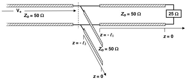
An open-circuit stub tuner is used to match the total impedance of the structure on the right (of the dashed line) to the 50  $\Omega$  impedance of the transmission line on the left carrying the input signal. You have at your disposal two design parameters - you can choose the lengths  $\ell_1$  and  $\ell_2$  of both the transmission lines.
