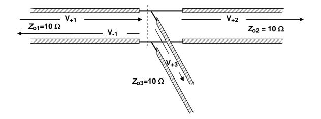
a) Looking to the right of the dashed line, the two output transmission lines can be represented as lumped impedances so the equivalent circuit becomes as shown below:
