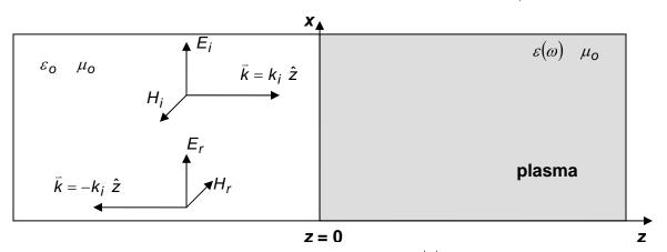
a) The frequency below which a wave is completely reflected (i.e.  $|\Gamma| = 1$ ) at the surface of a plasma is called the cut-off frequency  $\omega_c$ . In the previous homework you essentially showed that the cut-ff frequency  $\omega_c$  is just the plasma frequency  $\omega_p$  provided the wave is incident normally on the plasma. Now suppose a TE-wave is incident at an angle of incidence  $\theta_i$  as shown in the figure below.
