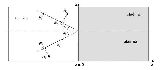
Find the cut-off frequency  $\omega_c$  as a function of the angle of incidence  $\theta_i$  for the TE-Wave. Is the cut-off frequency  $\omega_c$  now larger or smaller than the plasma frequency  $\omega_p$ ? **Hint:** think what is required to get  $|\Gamma| = 1$ . Although this problem is not about total internal reflection, you may want to study carefully how  $|\Gamma|$  becomes unity in the case of total internal reflection.
