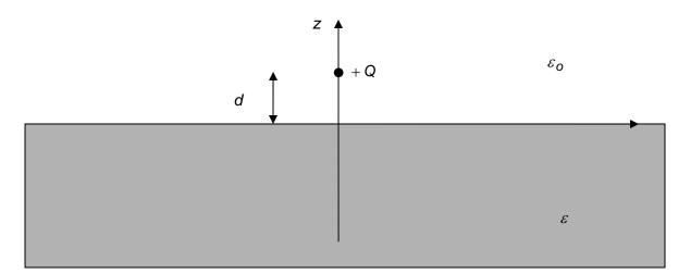
In this problem you will explore the forces exerted by dielectric interfaces on charges. As you have already seen in homework 3, charge density due to paired charges at can exist at dielectric interfaces and this charge density can also exert forces.
