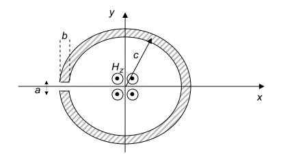
b) Now consider a conductive wire (not a perfect-metal wire) in the form of a loop. A magnetic field pointing in the +z-direction passes through the center of the loop as shown below. The magnetic field is time varying and the magnetic flux through the loop is a function of time and is given by the expression:  $\lambda(t) = gt$
