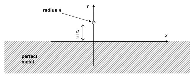
d) Find the inductance per unit length L (units: Henry/m) between the metal wire and the ground plane by taking the ratio of the magnetic flux per unit length (calculated in part (c) above) to the current I.
