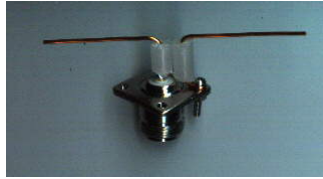
A 1-5 GHz home-made dipole antenna for Wireless LAN with a co-axial SMA RF feed
