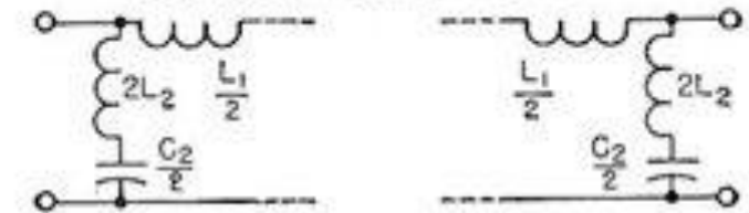
m -derived end sections for use with intermediate T section
